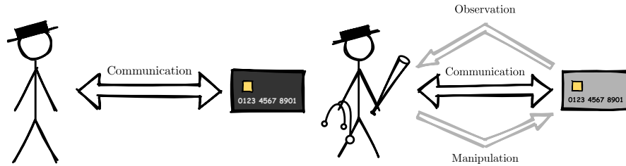
(a) Black-box security: A typical attack setting for cryptanalytic attacks. (b) Gray-box security: A typical attack setting for implementation attacks.
